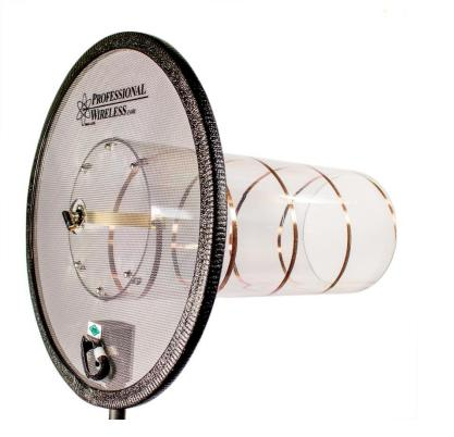
**SPECIFICATIONS RF Frequency Range / Bandwidth** 460 - 900 MHz Impedance 50 ohms Beamwidth 63 degrees **Antenna Gain** 10-12 dBi (on axis) Front-to-Back Ratio / Rear Rejection 12 dB **RF Connector** BNC female, right angle **Dual Mounting Adapter** 5/8"-27 U.S. standard 3/8"-16 European standard **Construction Material Clear Polycarbonate**
