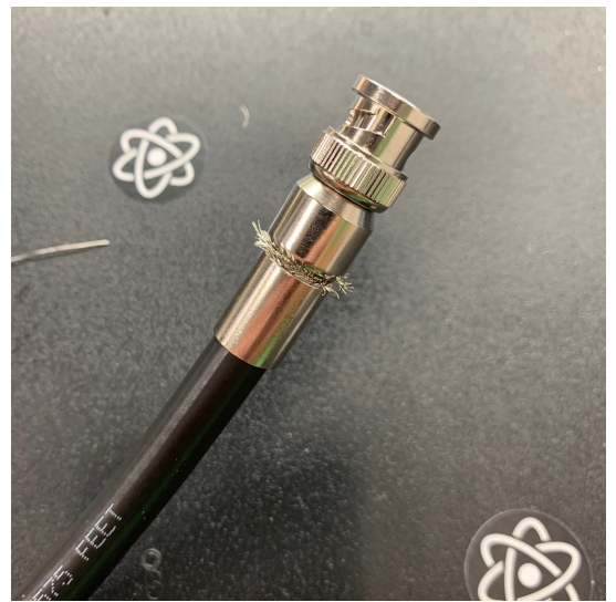
Slide the crimp sleeve over the braided shield to see how much excess needs to be trimmed.
