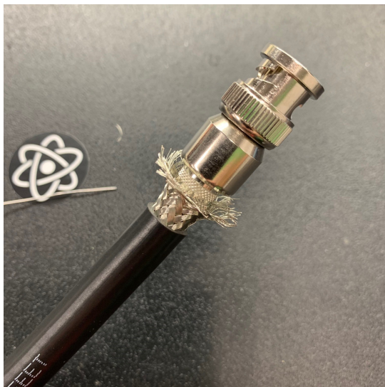
Carefully slide connector body over foil shield until the center pin clicks into position. Be sure the foil does not slide down the dielectric.
